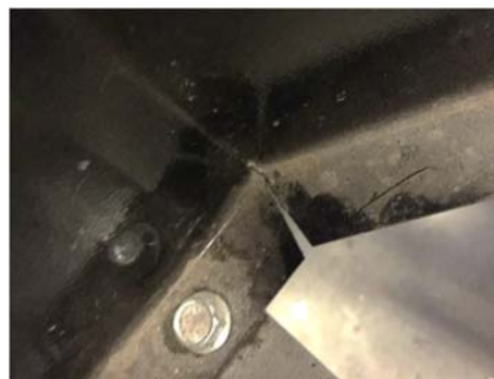
Figure 13. Stress concentration in sharp corner
