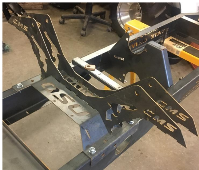
Figure 31. Test fit of the removable suspension structure
