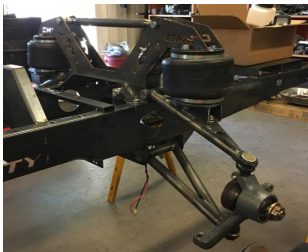
Figure 32. Suspension travel and alignment testing
