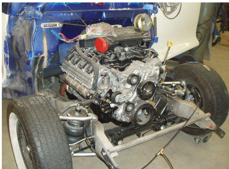
Figure 10. Example of air springs on a vehicle, from Progressive Automotive
