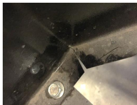
Figure 13. Stress concentration in sharp corner
