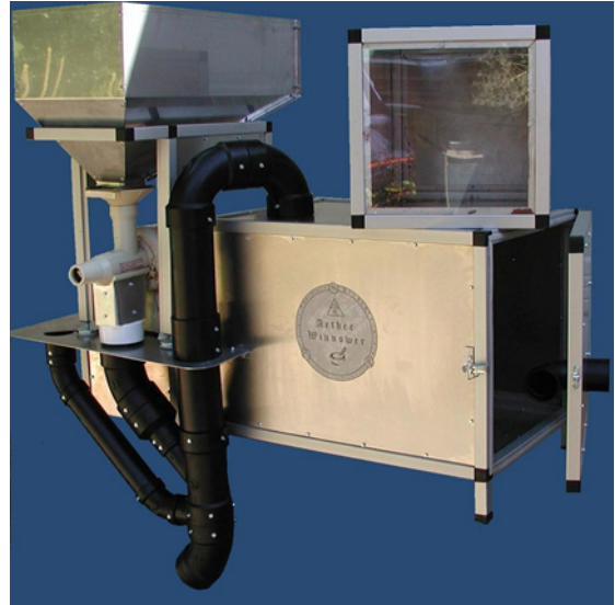
Figure 1.1 A photo of the Aether Winnower equipped with champion juicer
