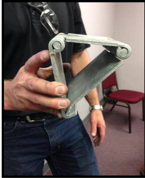
Figure 32 shows the lock desing, provided by Barrett Trailers.
