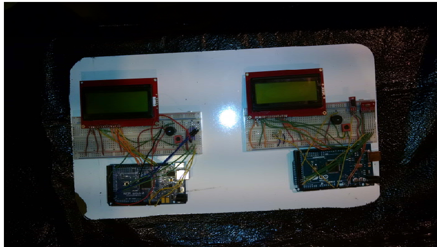
Figure 12: The two LCD displays for the Environmental Sensors that were installed in the full-scale analog.
