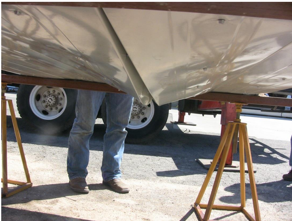
Figure 27: Deflection Along the Panels
