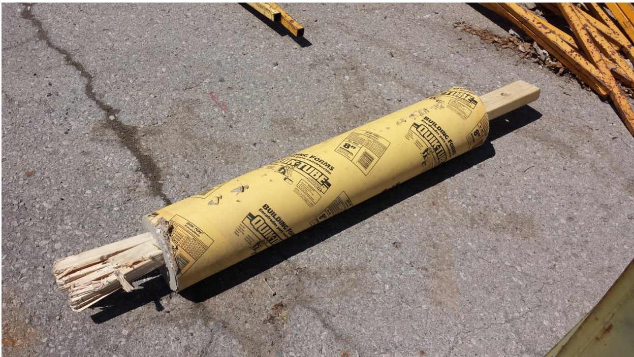
Figure 29: Missile Damage after Dropping
