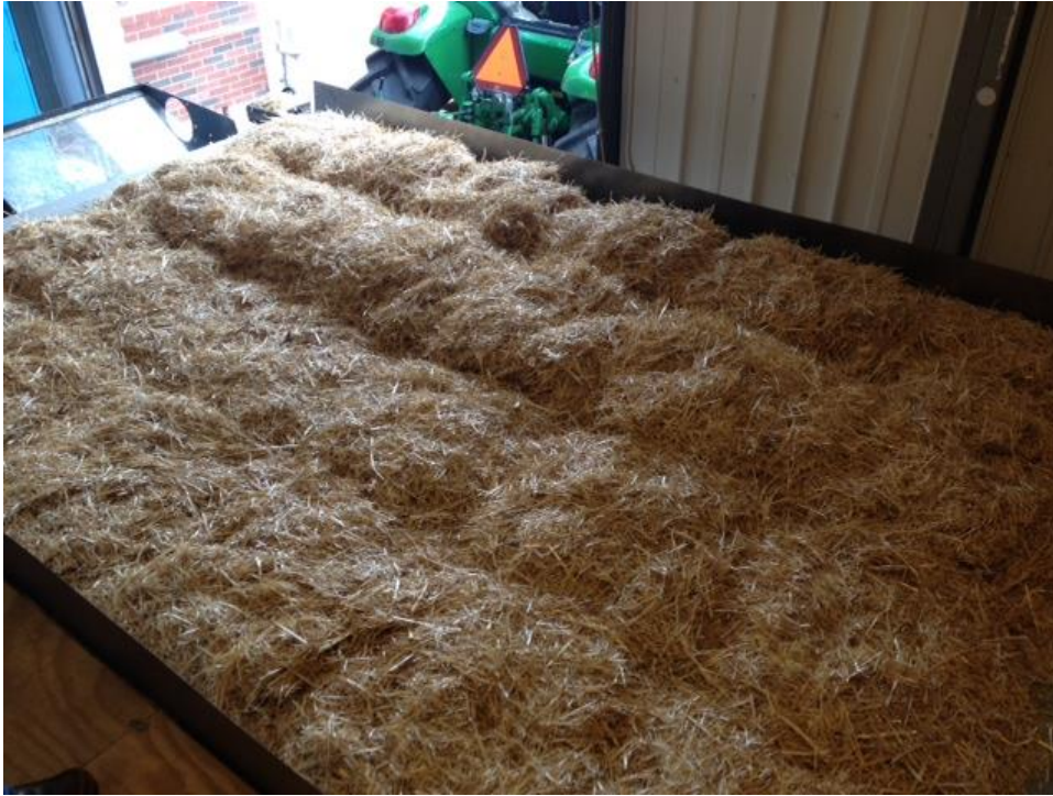
Figure 3: Material Conveyor system loaded evenly.
