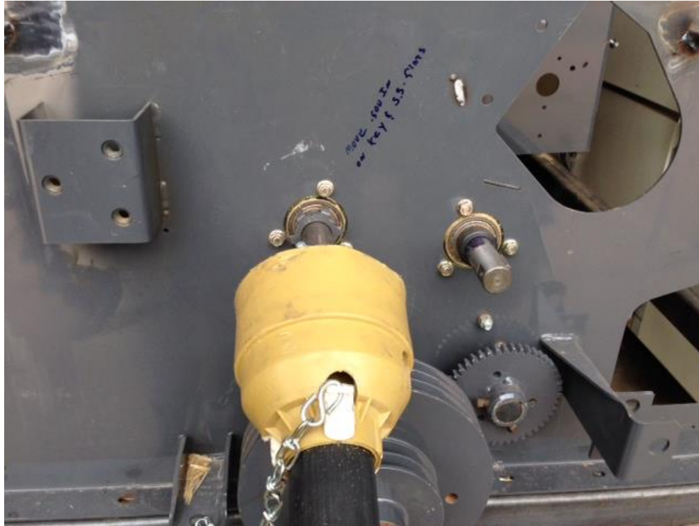
Figure 7: PTO powering the rear distribution auger
