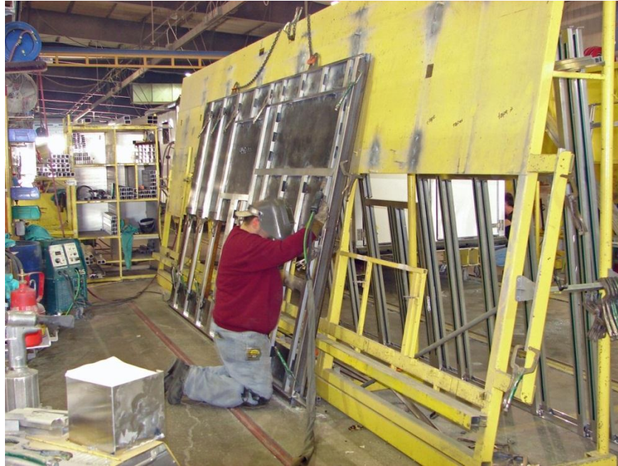
Figure 2 - Featherlight trailer side frame jig (Featherlite, 2009)
