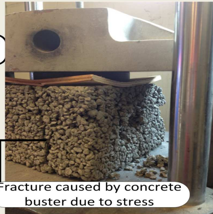
Figure 2 (Right): This shows block 6, which had undergone 35 freeze thaw cycles, being tested by the concrete buster. The image highlights a stress fracture on one side
