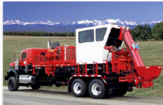
MC-60 Bodyload fracturing blender with closed chamber mixing system.
