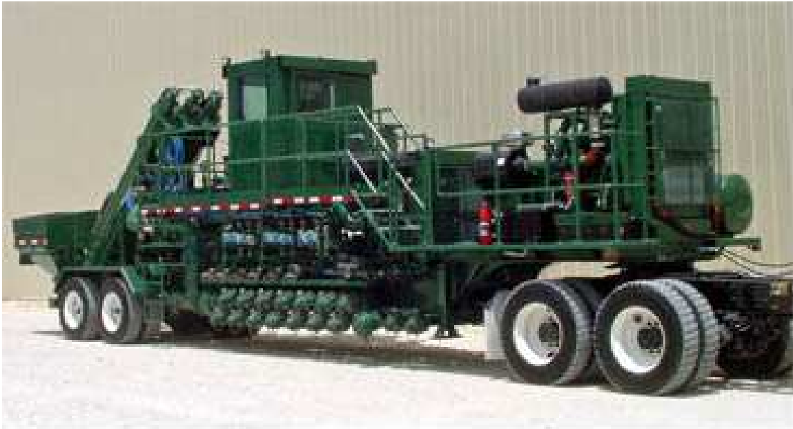
MT-1060 Blender equipped with eight (8) precision chemical metering systems
