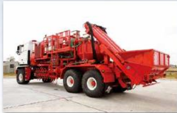
MC-60 Bodyload fracturing blender for extreme cold weather operations.
