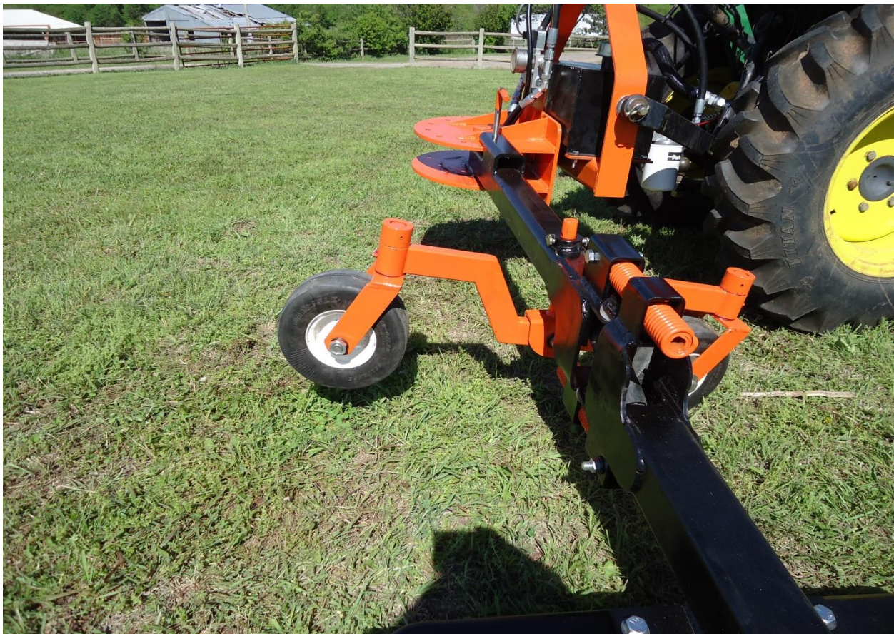
Figure 14 - This is a picture of the walking axle tilted to the front.
