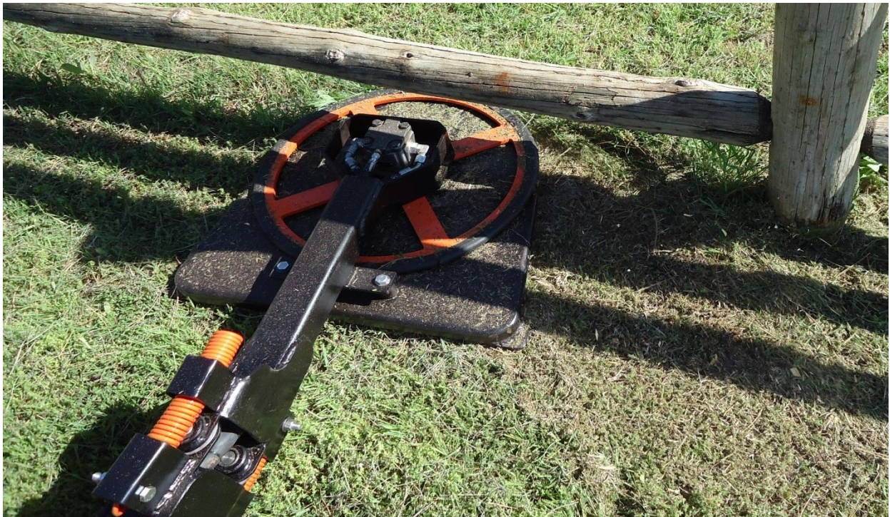
Figure 13 - The cutting head in position 4 right after the breakaway.
