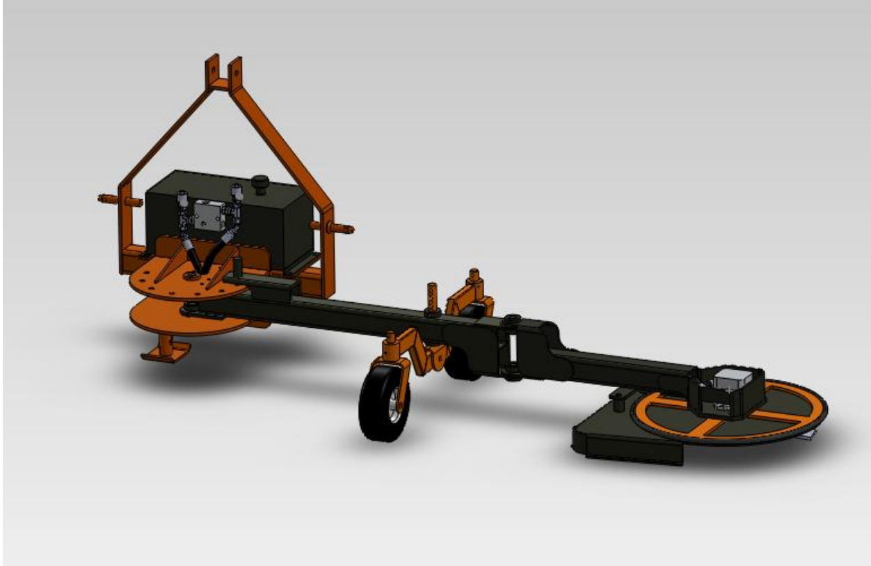
Figure 2 - Final CAD Design.
