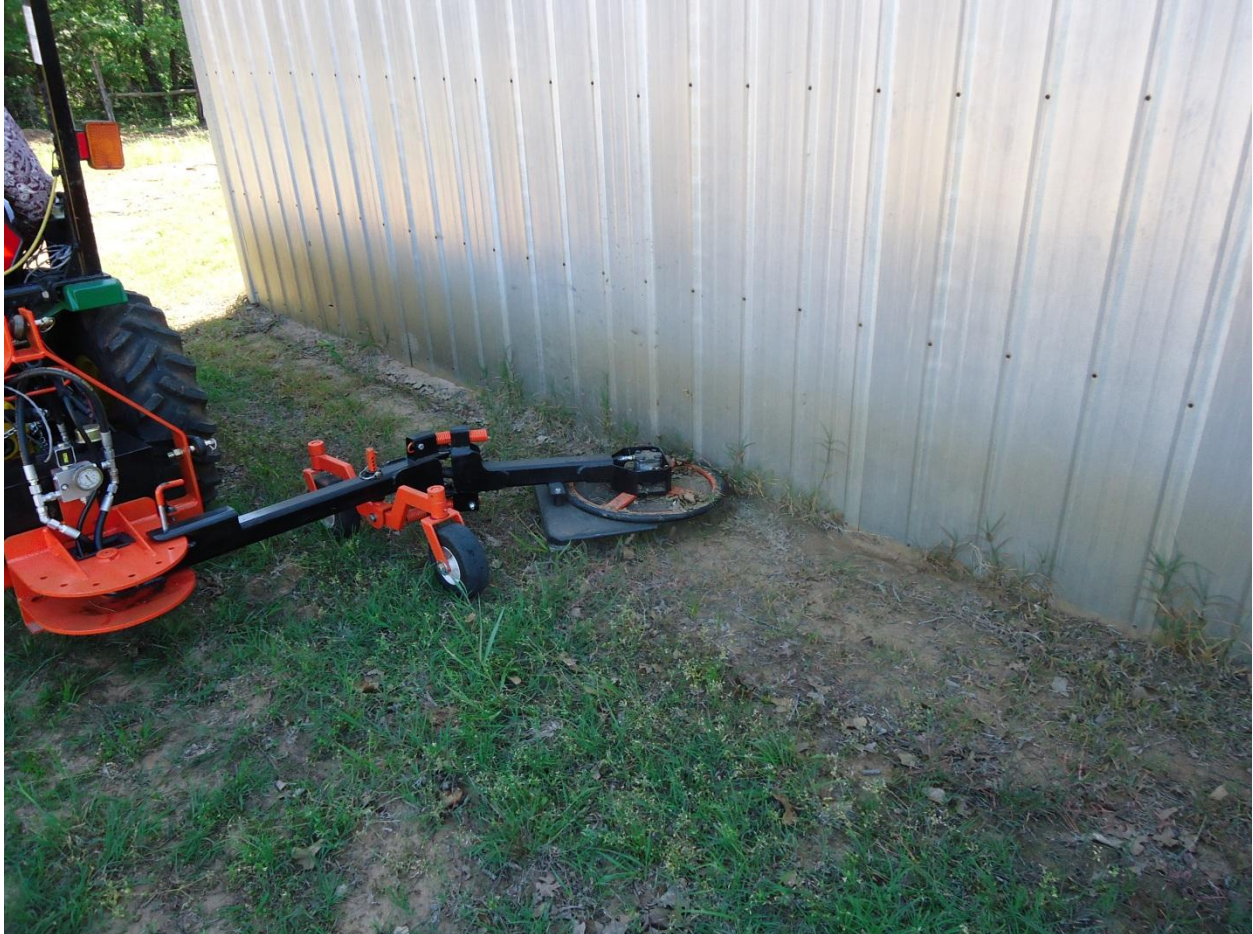
Figure 22 - This picture shows the working hinge working around a building.
