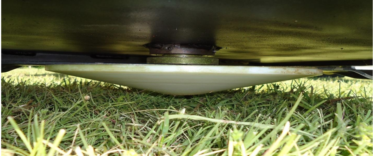
Figure 17 - This is the standard rotation dome for either a lawn mower blade or a disc mower blade.
