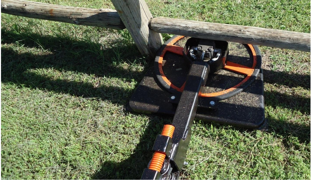
Figure 10 - This is the cutting head in position 1 right before breakaway.
