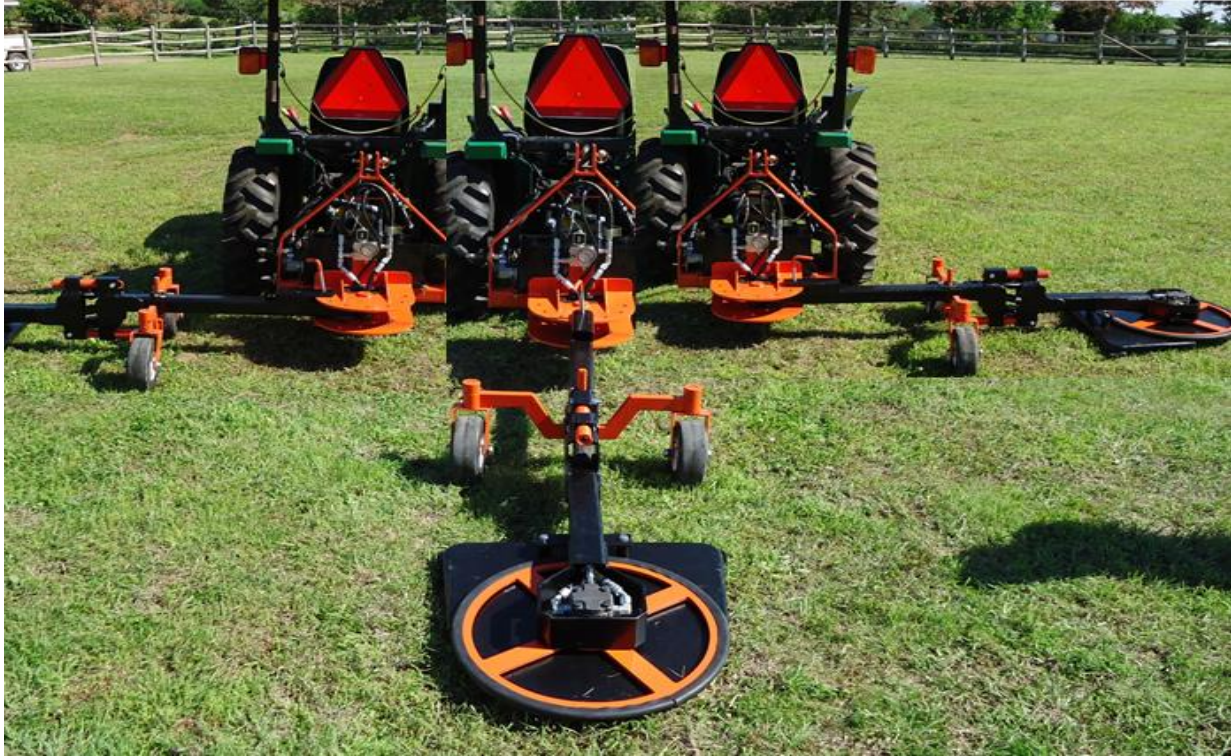
Figure 9 - This picture shows the indexing ability of the LTP.
