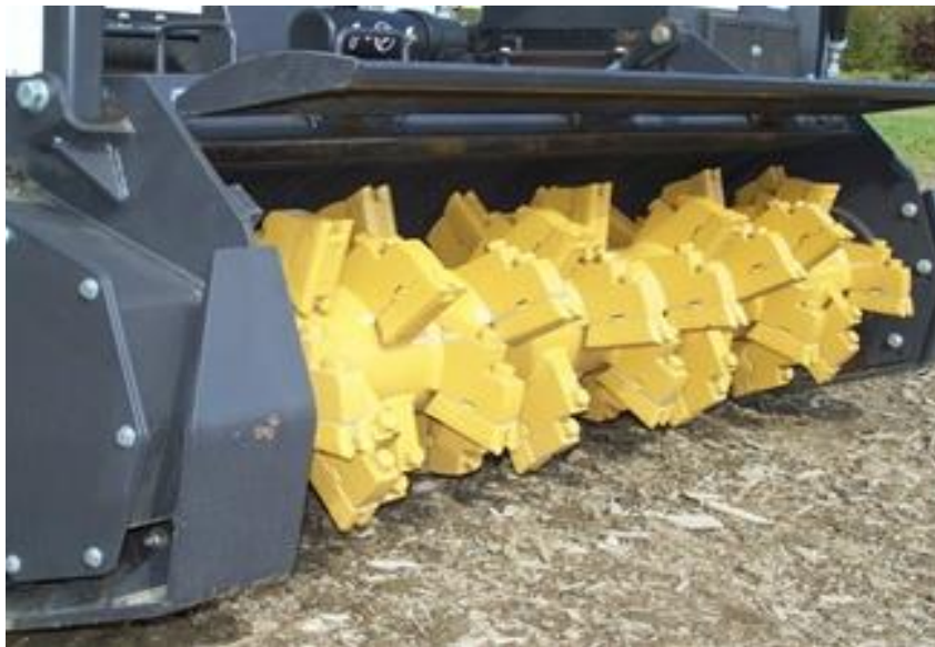
Figure 5. Mulcher Design Commonly Used for a Skid Steer
