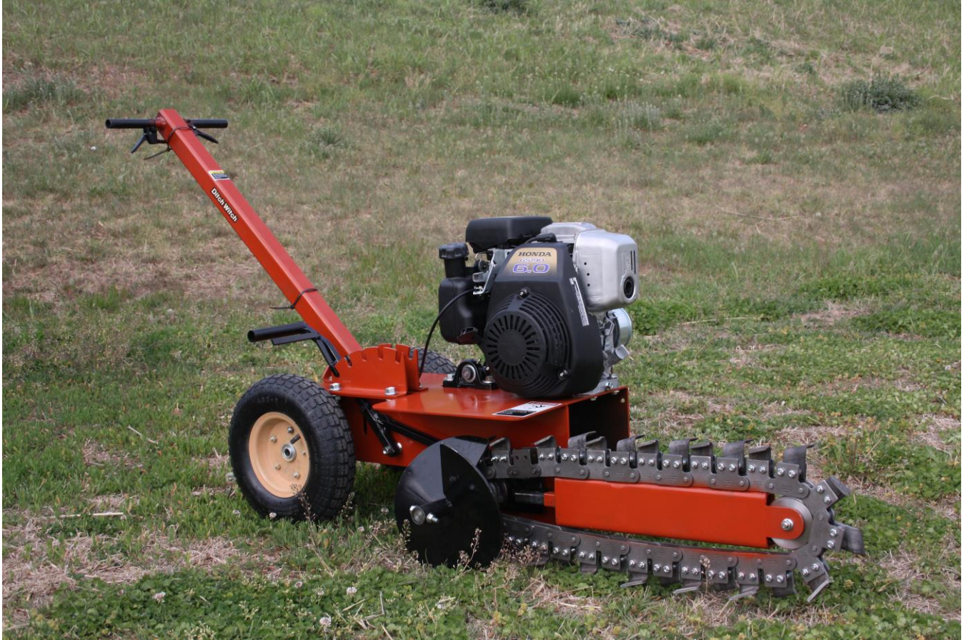
Figure 6: This figure shows the real prototype of the PT5 Walk-behind Trencher.
