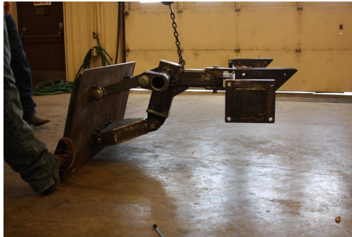
Figure 10. Four link system
