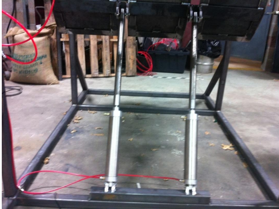
Figure 17. Pneumatics System Connected to the Drum Door
