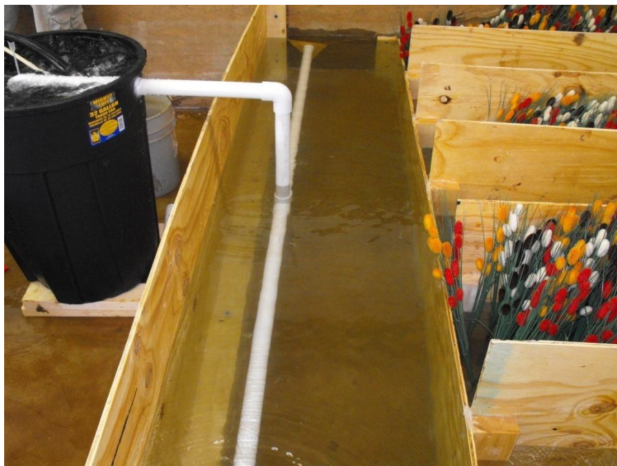
Figure 18 The overflow flow from the mixing tank was piped to the settling basin of the mesocosm structure. The pipe provided distributed flow along the width of the settling basin.
