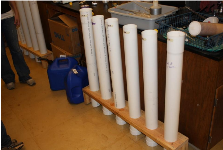
Figure 4. The Settling Tubes in which the jar tests were conducted. Alum was allowed to settle with time in the Illinois River filled tubes and samples were taken at different depths. The concentration of alum was varied.
