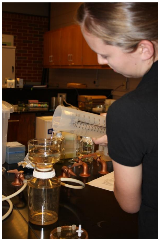
Figure 5. A vacuum filtration device was used to separate the suspended solids from the water. The filter was then weighed and recorded.
