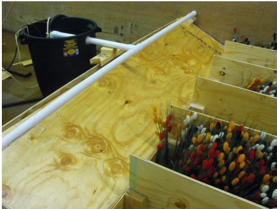
Figure 21. For the third and final test, the mesocosm structure was modified to bypass the initial settling basin. This allowed Scenic Solutions to examine the effects of the individual cells more thoroughly.
