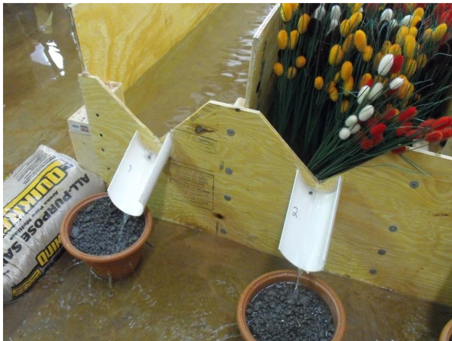
Figure 20. The water overflowed from the cells into the PVC discharge pipes into the slag baskets. Holes were drilled in the slag baskets to allow the water to drain. The water was then discharged.
