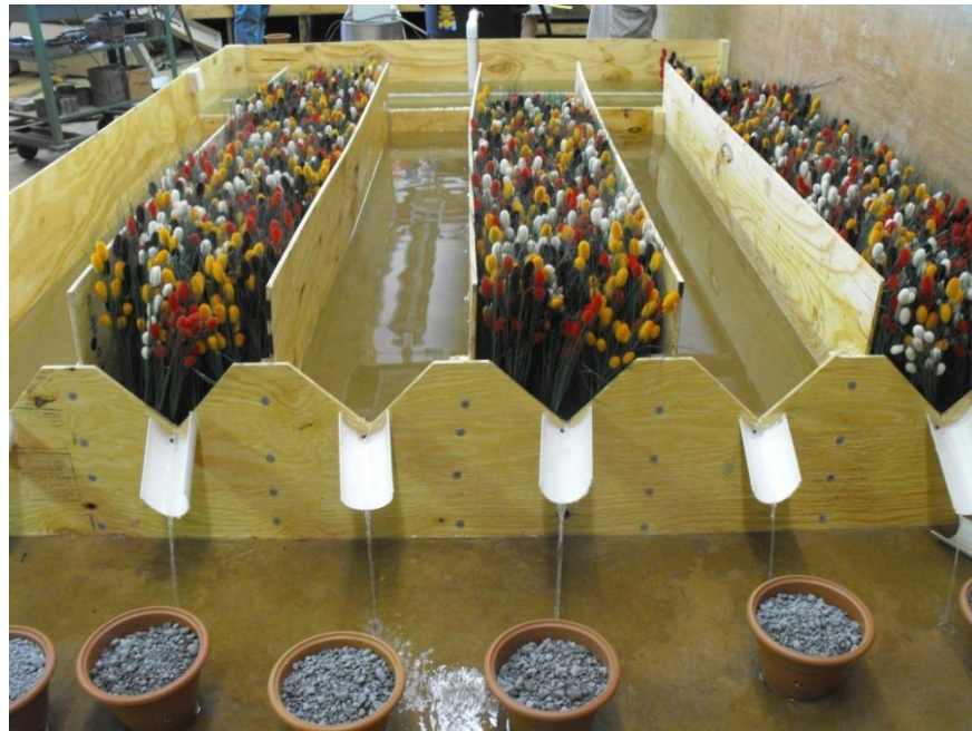
Figure 19. Water overflowed from the settling basin into the six mesocosm cells. Three of the cells were detention basins, and the other three provided the hydraulic characteristics of a wetland.
