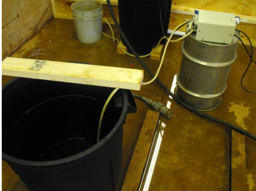
Figure 16. The concentrated alum was mixed with a known amount of Illinois River water and stored in the small black alum storage tank shown above. A peristaltic pump took this alum mix and pumped it to the mixing tank where it joined the Illinois River water.
