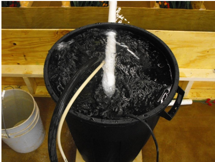
Figure 17. The alum mix and Illinois River water was mixed in the tank above. A submersible pump was dropped to the bottom of the tank to keep the water thoroughly mixed. The PVC then acted like an overflow device to drain the mixed water to the settling basin of the mesocosm.
