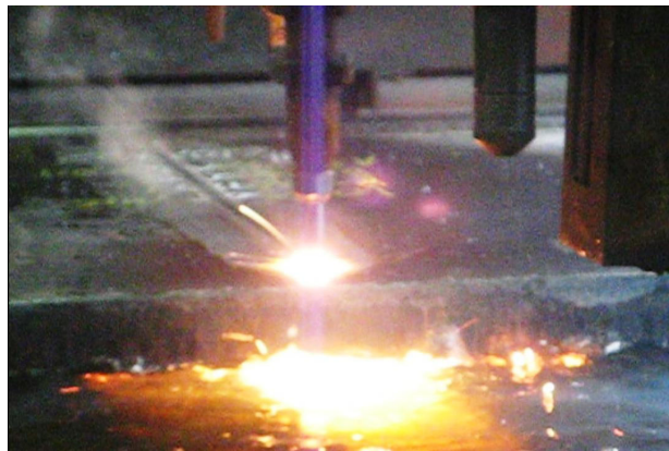
Figure 15: Blade Carrier Being Cut Out on Vassar Flame Table
