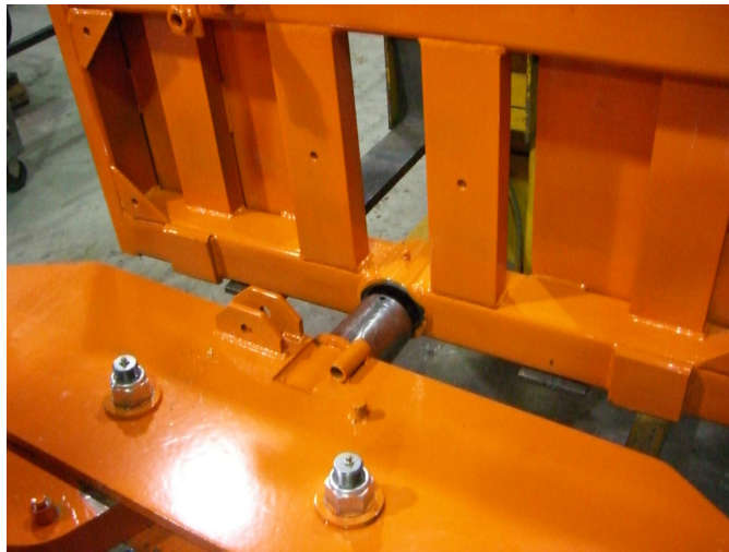
Figure 12: DOM Tubing for Rotation
