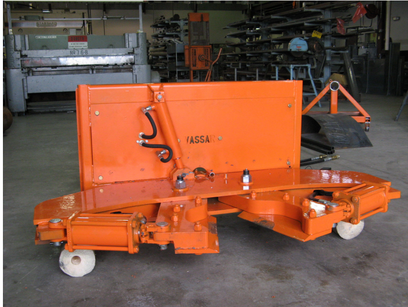
Figure 14: Assembled Tree Shear
