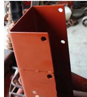
Figure 22: Pipe Box Extension
