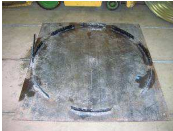
FIGURE 24 – METAL SLATS WELDED TO SUPPORT PLATE FOR INLET ATTACHMENT
