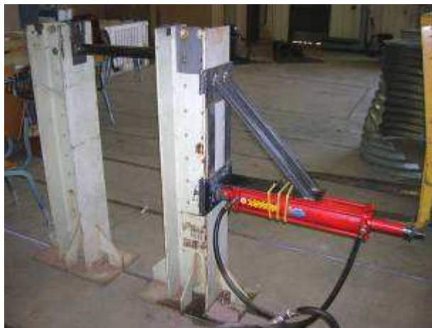
FIGURE 26 – SET-UP OF HYDRAULIC CYLINDER AND I-BEAM SUPPORTS
