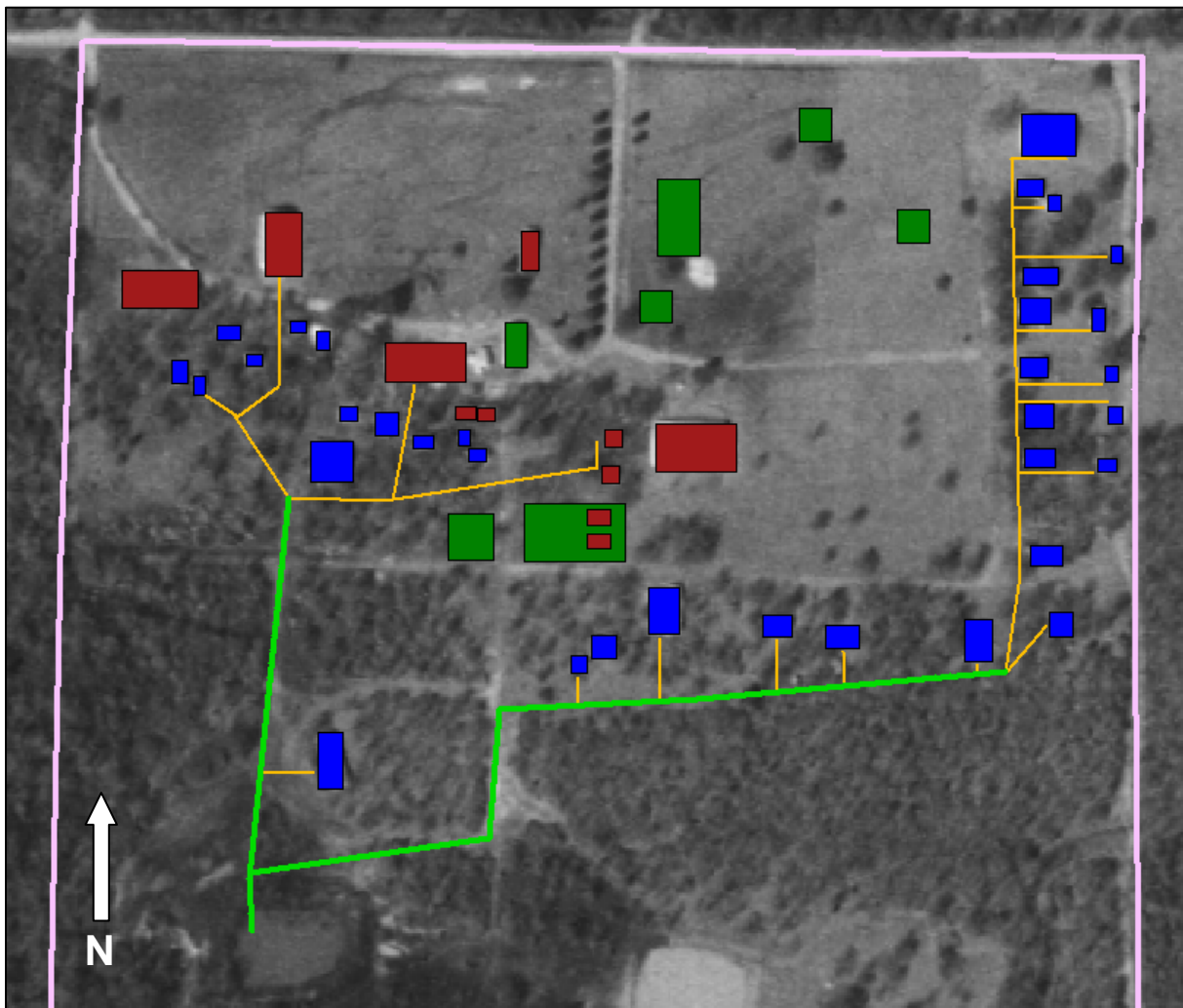
Figure 8. Sewer collection layout.
