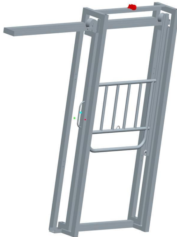
Figure 13. Guillotine/Slider Tail Gate
