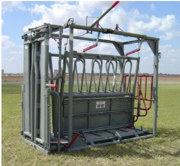
Figure 1. W-W Livestock System "BEEFMASTER" Current Chute Design
