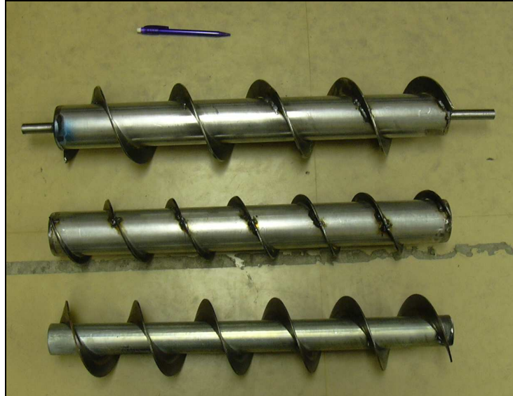
Figure 12: Fabricated Augers Exhibiting Various Flighting; auger #1 top, auger #2 middle, auger #3 bottom
