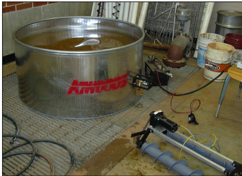
Figure 15: Testing Set-up displaying water and sand filled tank, load cell attached to tank, digital readout on chair, controller, and 12V DC battery.
