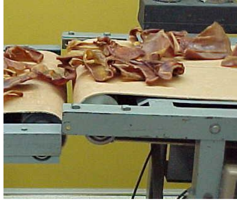
Figure 7: Different speed conveyors with an elevation difference
