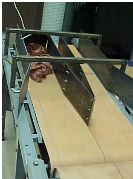
Figure 7: Trap door on the Lane Separating Device
