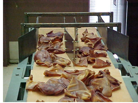
Figure 6: The actual Lane Separating Device
