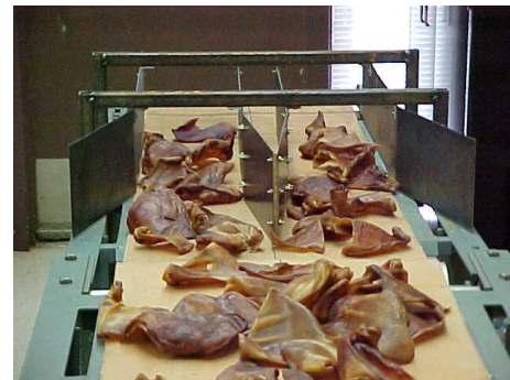
Figure 10: The actual Lane Separating Device
