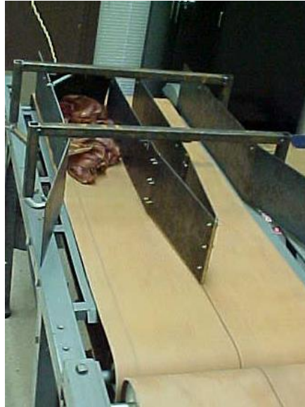
Figure 11: Trap door on the Lane Separating Device
