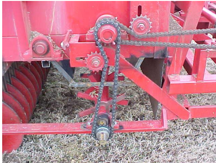
Figure 6: Spreader Bar Drive System
