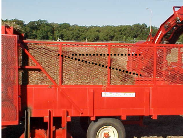
Fig. 3 Note the difference between the two dotted lines. The horizontal line is the desired sprig depth, while the diagonal dotted line illustrates the effects of the sprigs sloughing off of the back of the pile.
