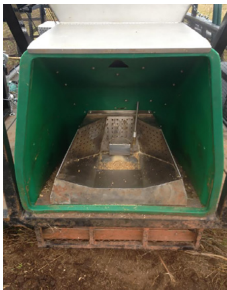
Figure 1. A) The head-box where animals receive the bait feed and gas emissions are collected. B) Profile view of the GreenFeed.
